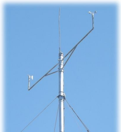
Typical installation on anemometric stations conforms to IEC61400-12
