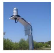
The installer will check that the height of the mast does not exceed the level of the pyranometer, to avoid measurement errors caused by reflections and shadow of the mast. It's recommended that pyranometer were thermically insulated from his bracket ensuring that there were a good electrical contact to ground.
