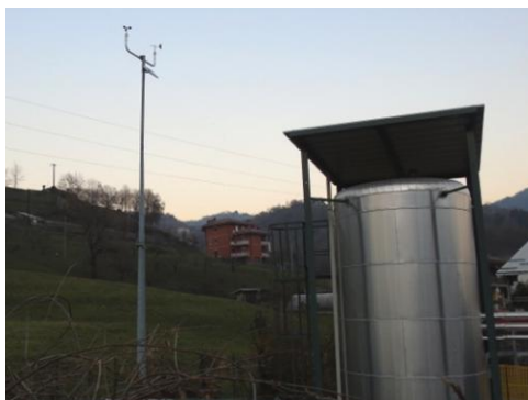
Meteorological station with 10m pole for monitoring of atmospheric pollutant dispersion (installation in cogeneration plant)
