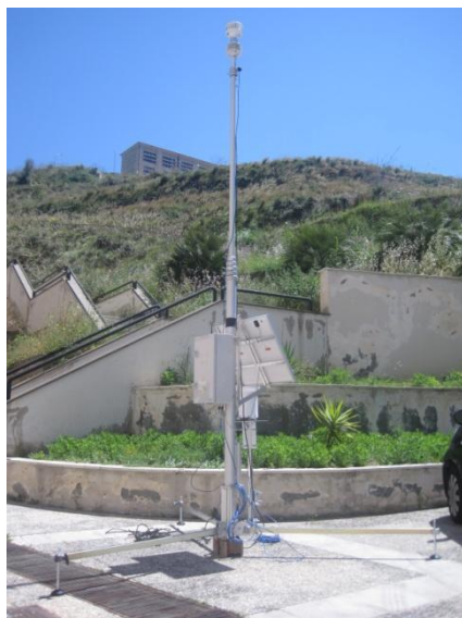
Meteorological portable station with 10m pneumatic pole, folding tripod and multi-parametric sonic anemometer with on-board compass
