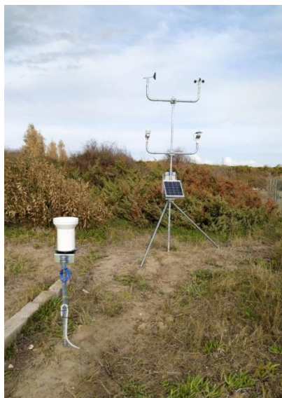
Weather station on telescopic pole h=3m (without civil works) for climatologic monitoring in the Taranto gulf
