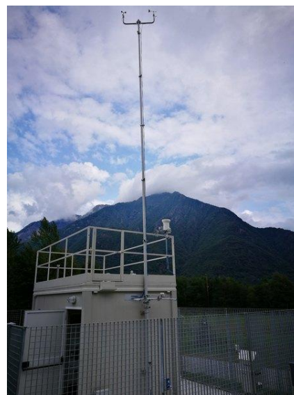
Meteorological station mounted on 10m light telescopic pole. Installation in a shelter for air quality analysis
