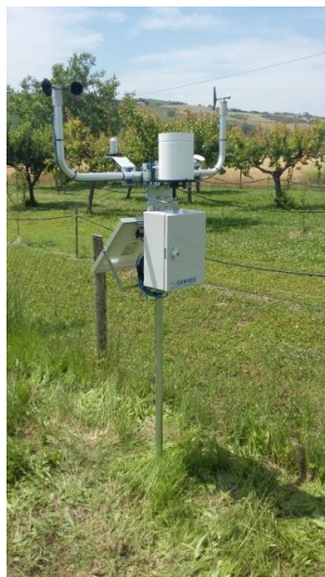
PF2-40 – Light pole h=2m with screw tip mounting (without civil works)
