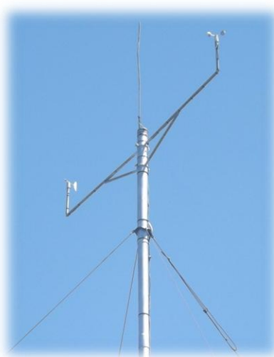
Typical installation on anemometric stations conforms to IEC61400-12
