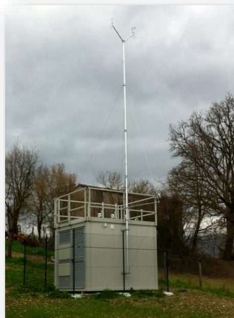
PTAP10-80 Meteorological pole h=10m compliant to WMO for environmental monitoring applications
