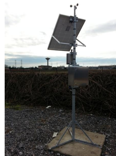
PF3-TREP – Heavy pole h=3m with foldable tripod and mounting on plinth or soil
