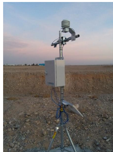
PL2-TREP – Light telescopic pole hmax=2.2m with tripod, fixing with ground stakes or concrete plugs
