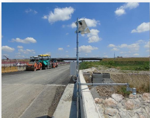
PF3-55 Telescopic pole h=3m for hydrometric applications
