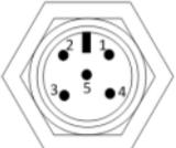
Pin1: Vout+<br>Pin2: Vout-<br>Pin3:<br>Pin4: Gnd<br>Pin5: +Vref. 1...24Vdc | Pin1: Iout+<br>Pin2:<br>Pin3:<br>Pin4:<br>Pin5: +Vdc 9...24Vdc | Pin1: Vout+<br>Pin2: Vout-<br>Pin3:<br>Pin4: Gnd<br>Pin5: +Vdc 9...24Vdc |
