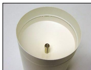
Internal view of the rain gauge filter and conic shape of rain collecting
