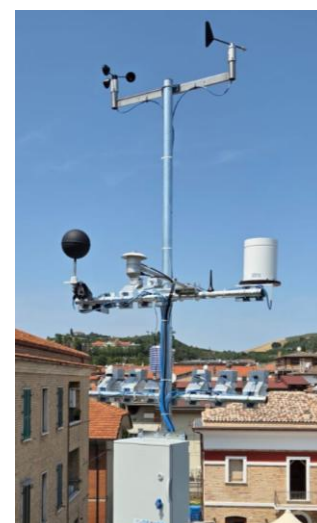
Rain gauge installation on pole with bracket cod. SBS2D
