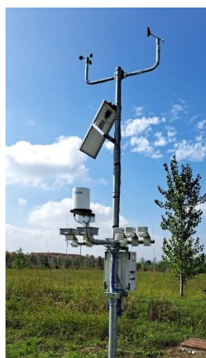
Rain gauge installation on pole with L bracket cod. SPL-L
